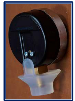
Step 7: Rubber stopper correctly inserted into pressure gauge
